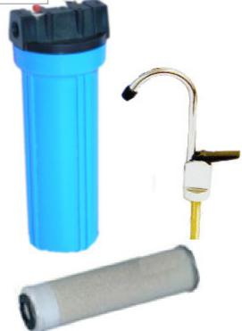
Penstar Point-of-Use Nitrate Filter Kit uses a 10" or 20" slimline filter housing with a nitrate selective resin cartridge to supply a separate drinking water tap.
