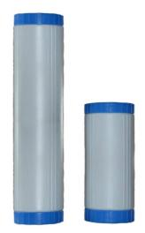
Penstar MRC cartridges, fitted in normal large diameter filter housings, provide simple, effective reduction of dissolved iron in domestic water supplies. Often will also reduce manganese levels to some extent but, in this case, performance cannot be guaranteed.
